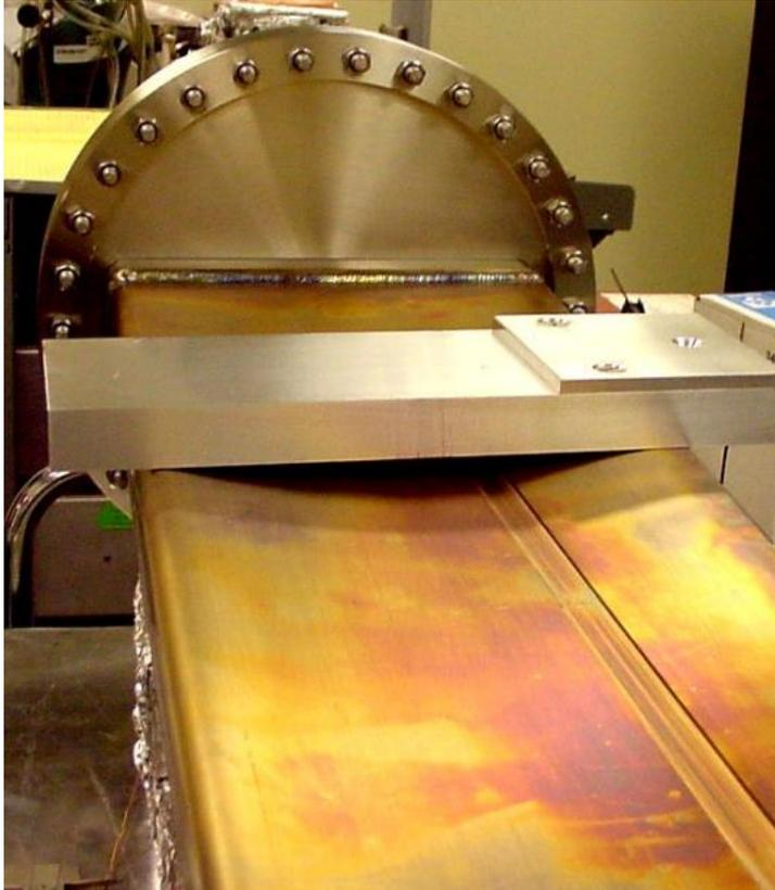
*Disformed copper chamber during a bakeout*
